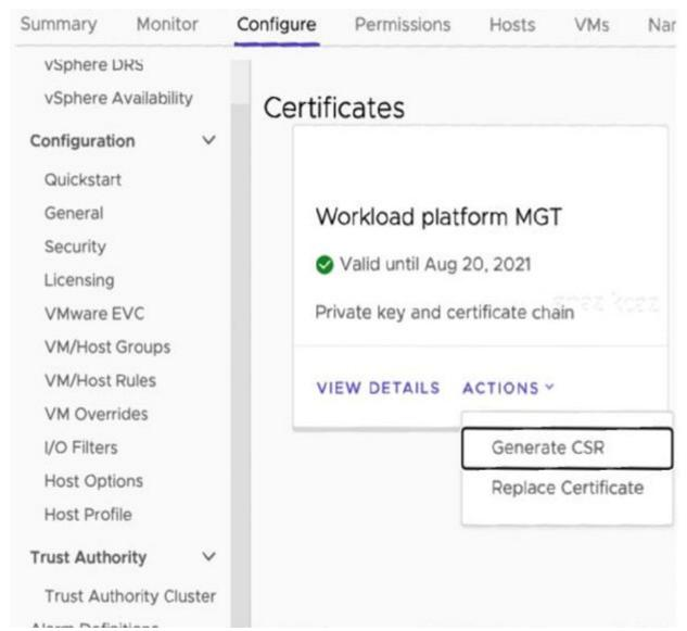
As a vSphere administrator, you can replace the certificate for the virtual IP address (VIP) to securely connect to the Supervisor Cluster API endpoint with a certificate signed by a CA that your hosts already trust. The certificate authenticates the Kubernetes control plane to DevOps engineers, both during login and subsequent interactions with the Supervisor Cluster.
