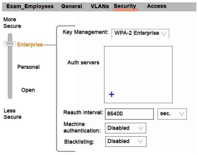
Network administrators need to set up a WLAN that uses WPA2 encryption and authenticates users with a preshared key (PSK) that is the same for all users. Administrators do not see where they should specify the option for the preshared key.
