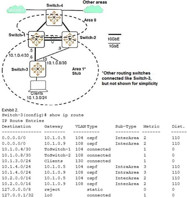
The exhibits show the current operational state for routes on Switch-3. The company wants Switch-3 to prefer the link to Switch-1 over the link to Switch-2 for all intra-area, inter-area, and external traffic. What can the network administrator do to achieve this goal?
