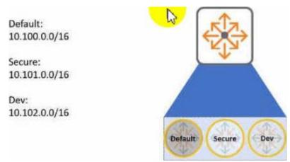
Aruba CX 6300 switch has routes in three different VRFs as per the example above. The user needs to leak routes between VRF Secure and VRF Dev. and also between VRF default and VRF Dev. The customer Is not able to establish routing between directly connected networks 10.100.50.0/24 and 10.102.26.0/24.
