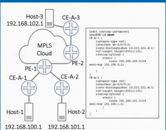
Referring to the exhibit, there is an Layer 3 VPN setup that connects sites CE-A-1. CE-A-2 and CE-A-3 together Host-1 can communicate with Host-3. but Host-1 cannot communicate with Host-2 What must you do to solve the problem?
