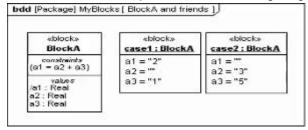
The modeler has set all shown values us inputs and next intends to solve the mode that is, to calculate the outputs. Assume nothing relevant has been left out.
