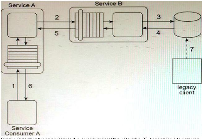
Service Consumer A invokes Service A in order to request this data value (1). For Service A to carry out this request, it must invoke Service B (2), a utility service that interacts (3, 4) with the database in which the data value is stored. Regardless of whether the data value changed, Service B returns the latest value to Service A (5), and Service A returns the latest value to Service Consumer A (6).
