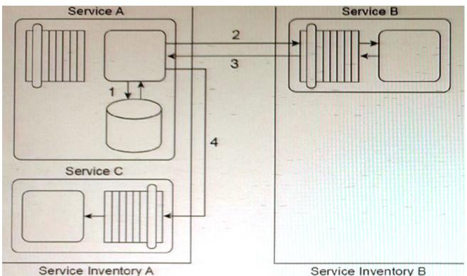
Before it contacts Service B, Service A must first retrieve a list of code values from its own database (1) and then place this data into its own memory. If it turns out that it must send a message to Service C, then Service A must combine the data it receives from Service B with the data from the code value list in order to create the message it sends to Service C. If Service A is not required to invoke Service C, it can complete its task by discarding the code values.
